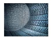
The firing method is the same as the barrels used for bourbon aging. Like the skin of a crocodile Carbonize until it becomes The thickness of the carbonized layer is approximately 4 mm.
